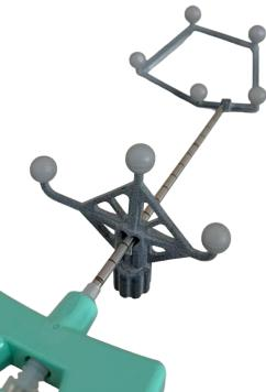
Slide the needle in the Needle fiducial - Sensor IR distal clip until a small portion of the needle tip is visible on the bottom of the Needle fiducial - Sensor IR distal clip. It is recommended to place Needle fiducial -Sensor IR distal clip on the patient in order to identify the best entry trajectory and to use rigid needles (introducers) in order to avoid needle bending during the insertion.
