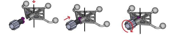
The operator can proceed with the calibration of the needle, placing the tip of the needle in the cavity of
